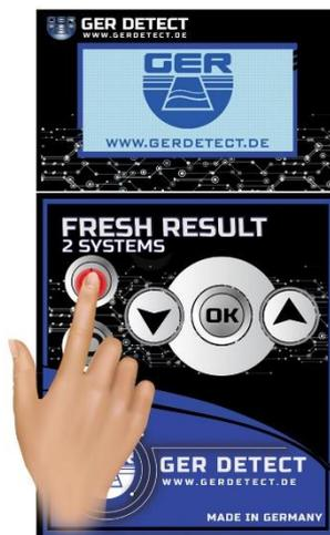
We turn the device through the power switch
